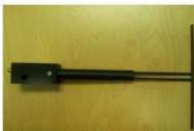
Figure 1 – MVG COMOSAR Validation Dipole
