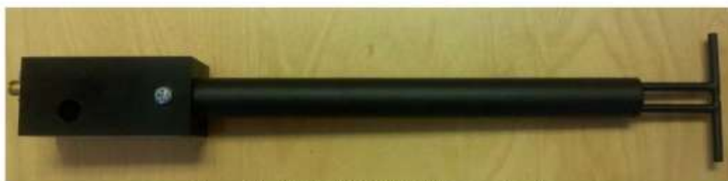
Figure 1 – MVG COMOSAR Validation Dipole
