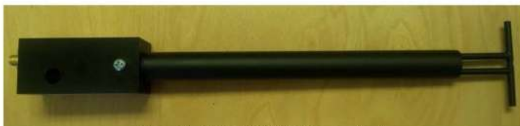
Figure 1 – MVG COMOSAR Validation Dipole
