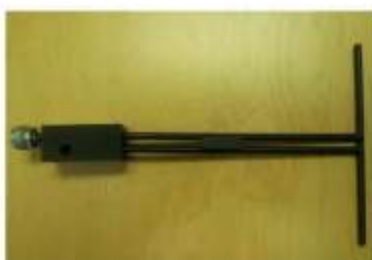
Figure 1 – MVG COMOSAR Validation Dipole
