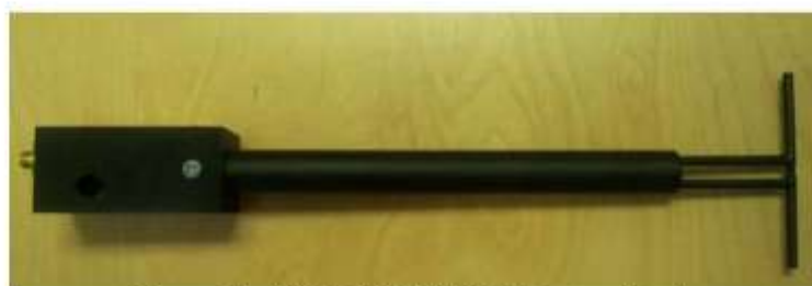
Figure 1 – MVG COMOSAR Validation Dipole
