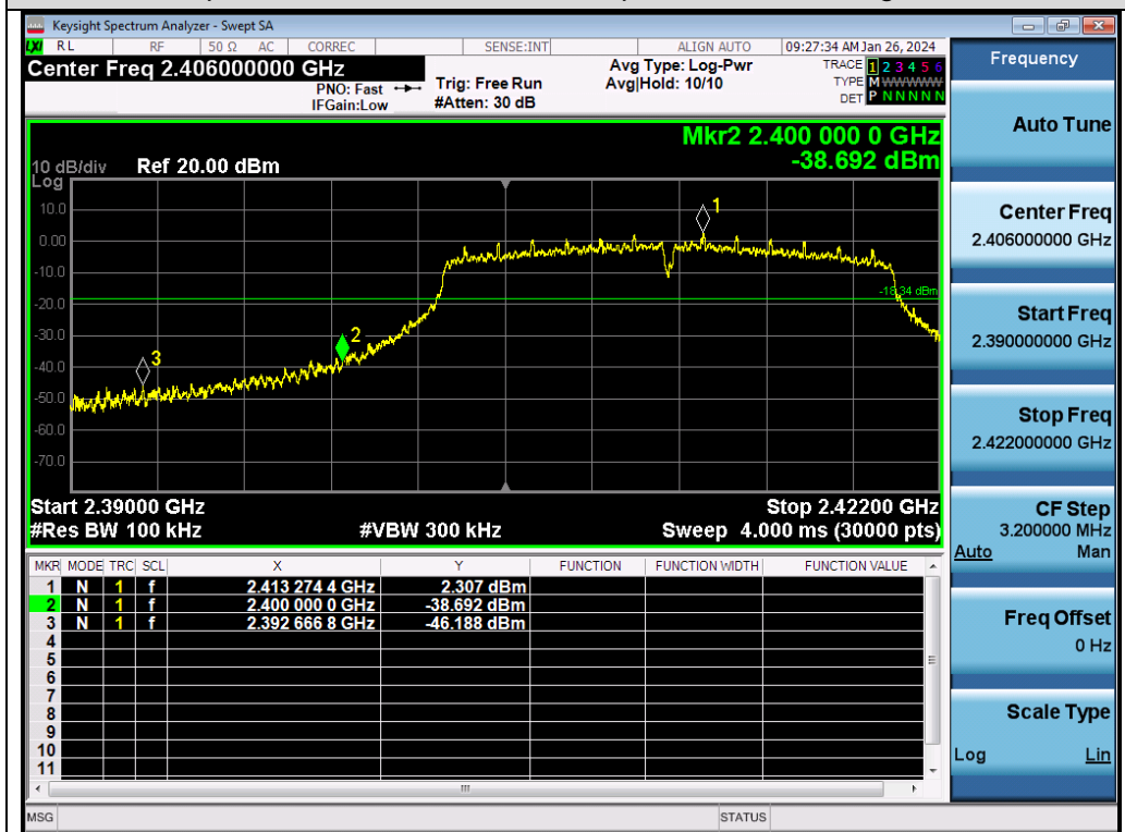
Test_Graph_802.11g_ANT1_2412_6Mbps_Lower Band Edge Emissions
