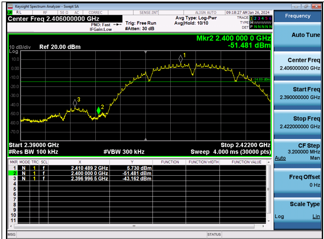
Test_Graph_802.11b_ANT1_2412_1Mbps_Lower Band Edge Emissions
