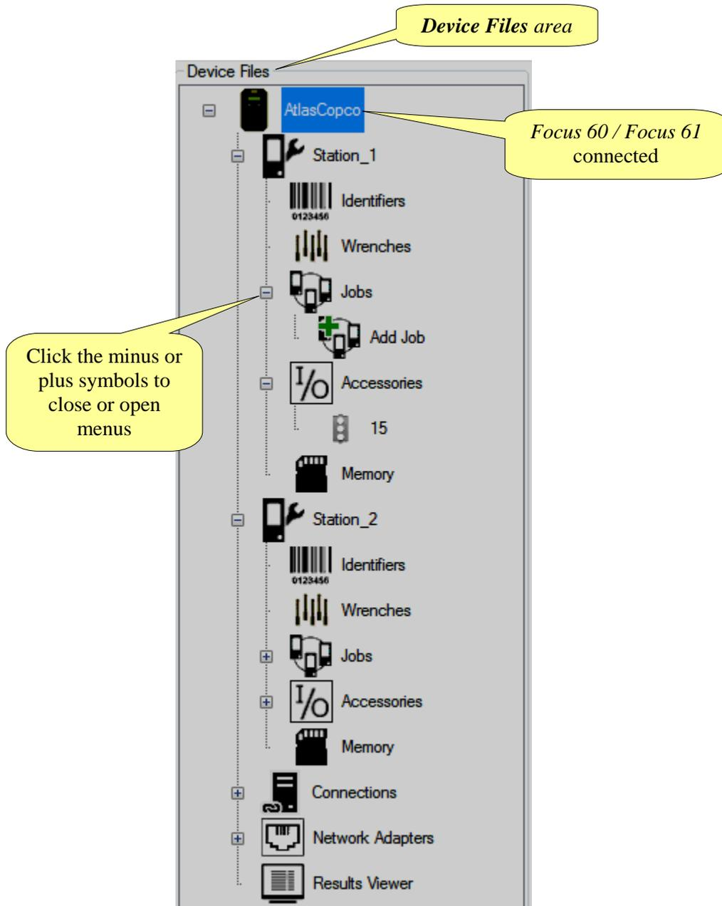
The *Device Files area* defines the stations associated with the *Focus 60 / Focus 61* connected. For each station there are MWR-TA associated, which execute the *Jobs* programmed.
