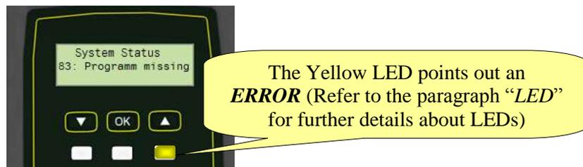
If a MWR-TA is associated with one Station of the *Focus 60 / Focus 61*, but either the batteries level of the MWR-TA is too low or the MWR-TA is out of the range of the *Focus 60 / Focus 61*, the following screen is shown:
