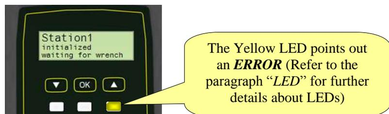
Associate the MWR-TA with a Station of the *Focus 60 / Focus 61*. After few seconds, the *Focus 60 / Focus 61* shows the data of the ongoing tightening operation on the MWR-TA (refer to the following picture):
