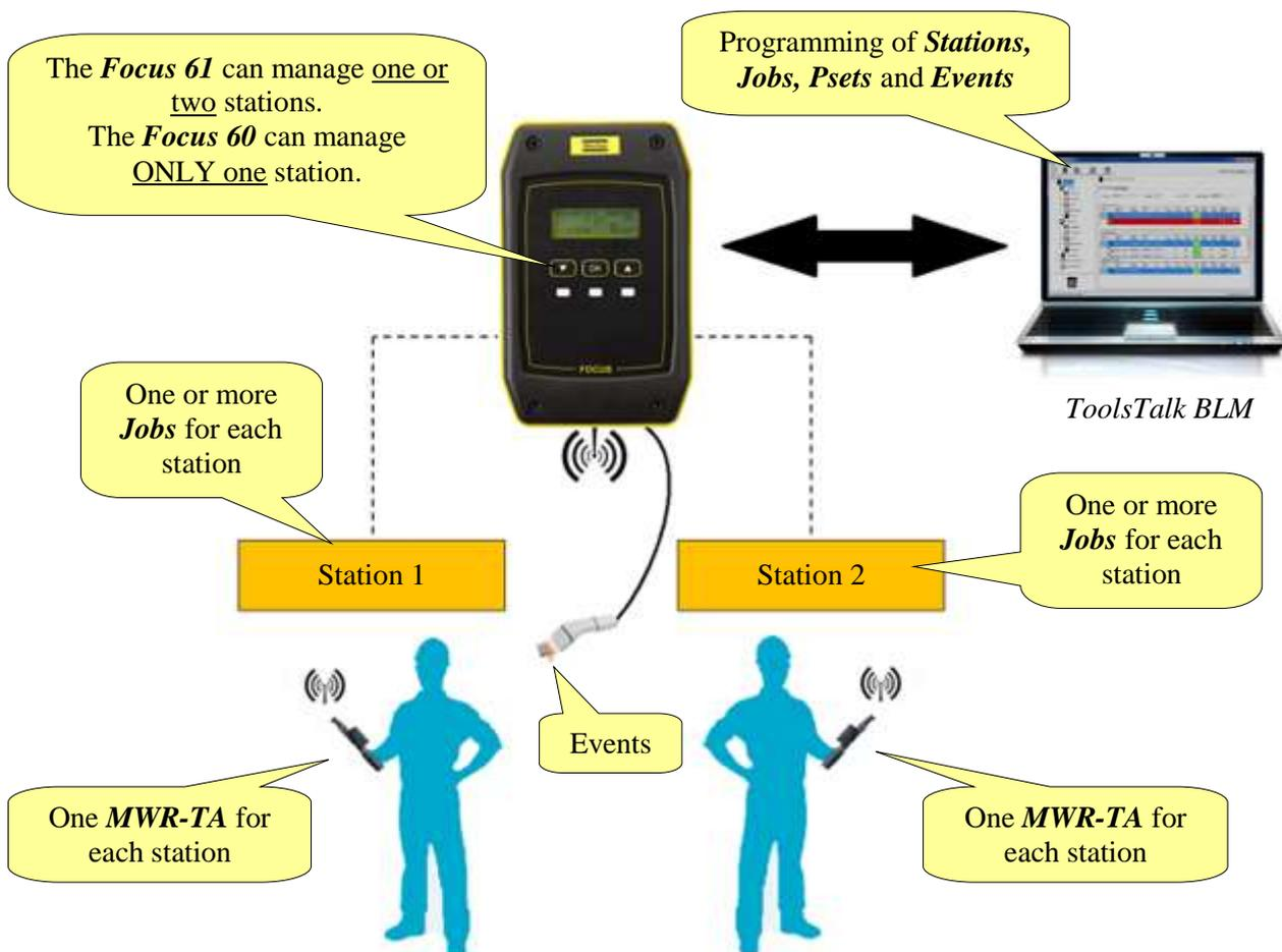
The *Focus 61* can manage one or two stations, while the *Focus 60* can manage only one station.
