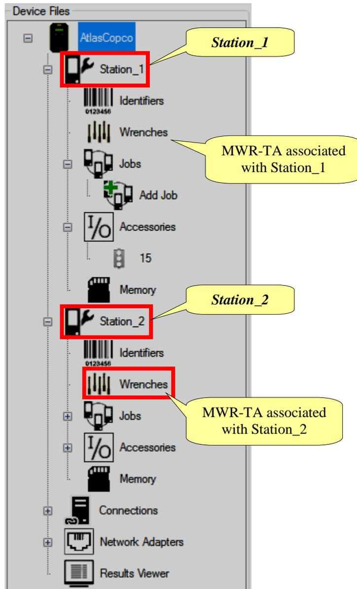
It is possible to associated up to 10 MWR-TA with a **Focus 61**, divided into the two *Stations* (one MWR-TA on one *Station* for **Focus 60**).
