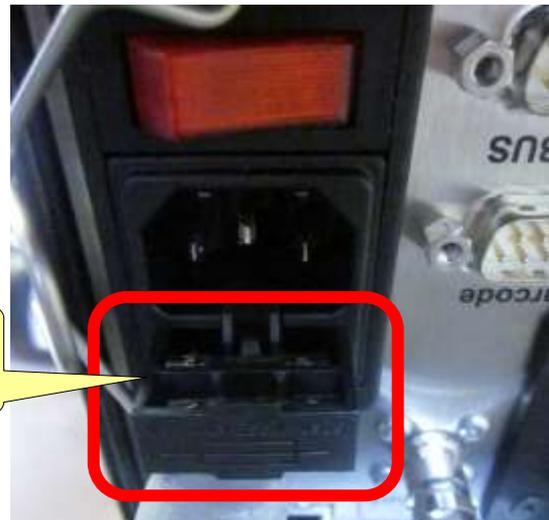
6. After installing the new *Miniature Fuses*, push the Fuses Holder into its housing as shown in the picture on the right:
