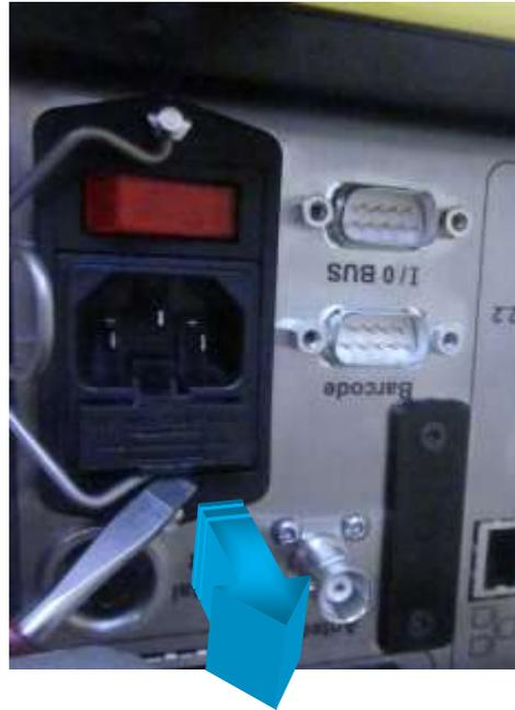
5. After extracting the *Fuses Holder*, it is possible to see the two *Miniature Fuses* (refer to the picture on the right).
