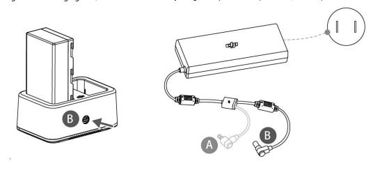
Tips: The charging hub can charge two batteries at the same time. It will take a longer time to charge the Intelligent Flight Battery and remote controller together.
