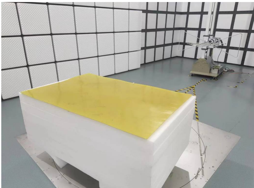
Photo of Radiated Emission Measurement (Above 1G)
