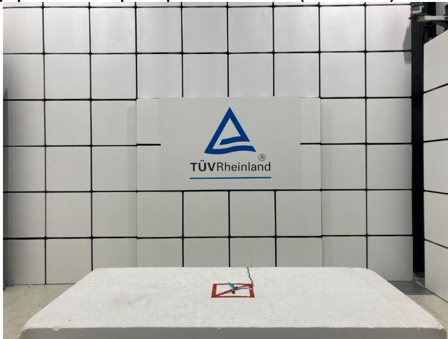
Photograph 2: Test Setup for Spurious Emissions (Front View 2)
