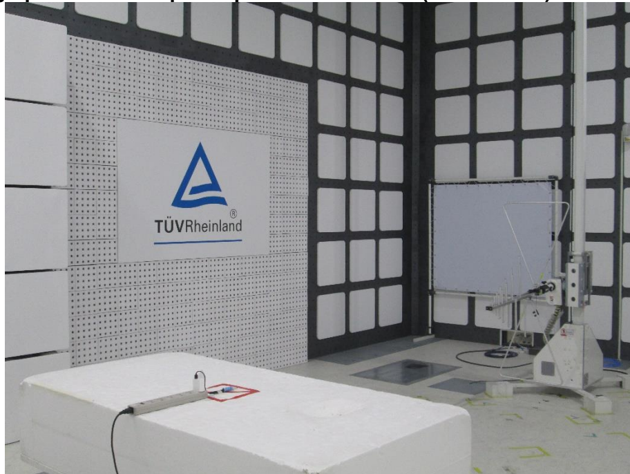
Photograph 9: Test Setup for Spurious Emissions (Back View 2)
