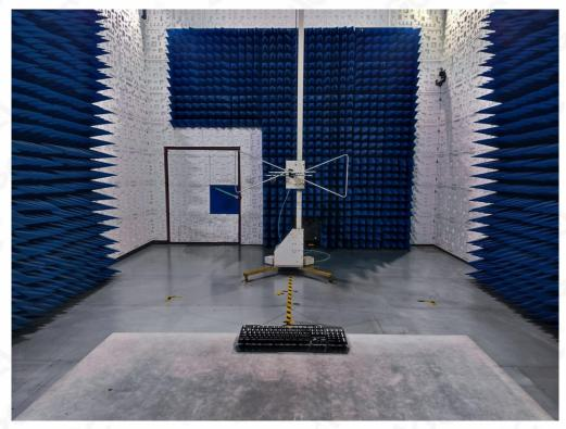
RADIATED EMISSION TEST SETUP ABOVE 1GHz
