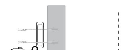
4. Place the baby unit on the wall mount bracket, and then slide it forward until it locks into place. Connect the power adapter to the baby unit and a power supply.
