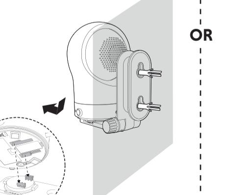
5. You can maximise your baby unit's viewing angles by tilting the wall mount bracket. Hold the baby unit, and then rotate the knob in an anticlockwise direction. This will loosen the joint of the wall mount bracket. Tilt your baby unit up or down to adjust to your preferred angle. Then, rotate the knob in a clockwise direction to tighten the joint and secure the angle.
