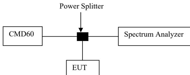
**Spurious radiated emission set up:**
