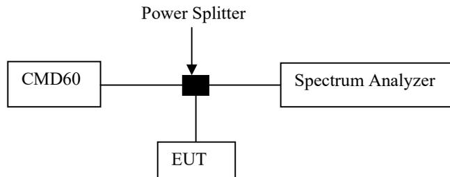
The width, in Hz, of the signal between two points, one below the carrier center frequency and one above the carrier center frequency, that is 26 dB down relative to the maximum level of the modulated carrier. It is based on the use of measurement instrumentation employing a peak detector function with an instrument resolution bandwidth approximately equal to 1% of the emission band-width of the device under measurement. [Extraction from 47 CFR 15, subpart D, 15.303 (C)].
