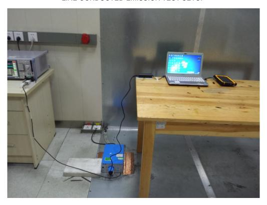
RADIATED EMISSION TEST SETUP
