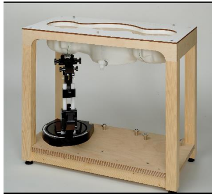
Picture C.10: SAM Twin Phantom
