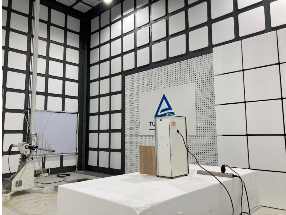
Photograph 3: Test Setup for Spurious Emissions (Back View 2)
