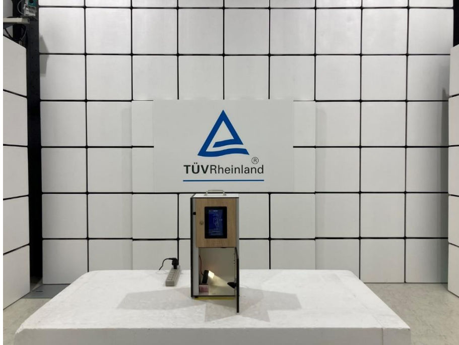
Photograph 1: Test Setup for Spurious Emissions (Front View 1)
