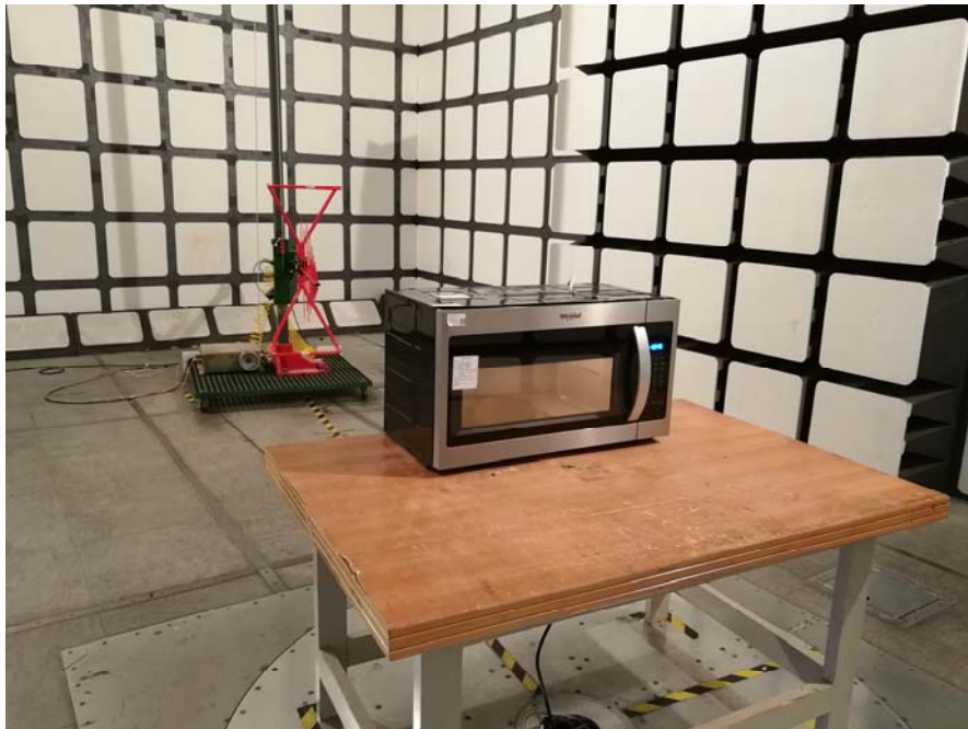
Radiated Emissions - Front View (30 MHz – 1 GHz)
