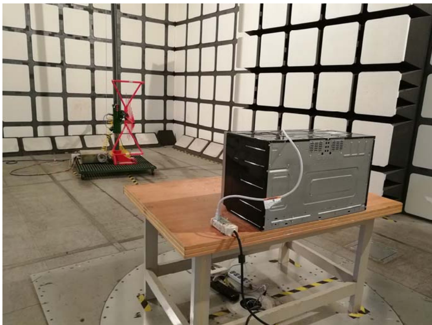
Radiated Emissions - Rear View (30 MHz – 1 GHz)
