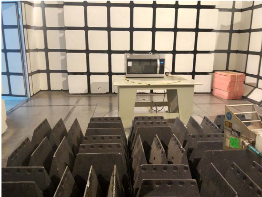
Radiated Emissions - Front View (Above 1 GHz)
