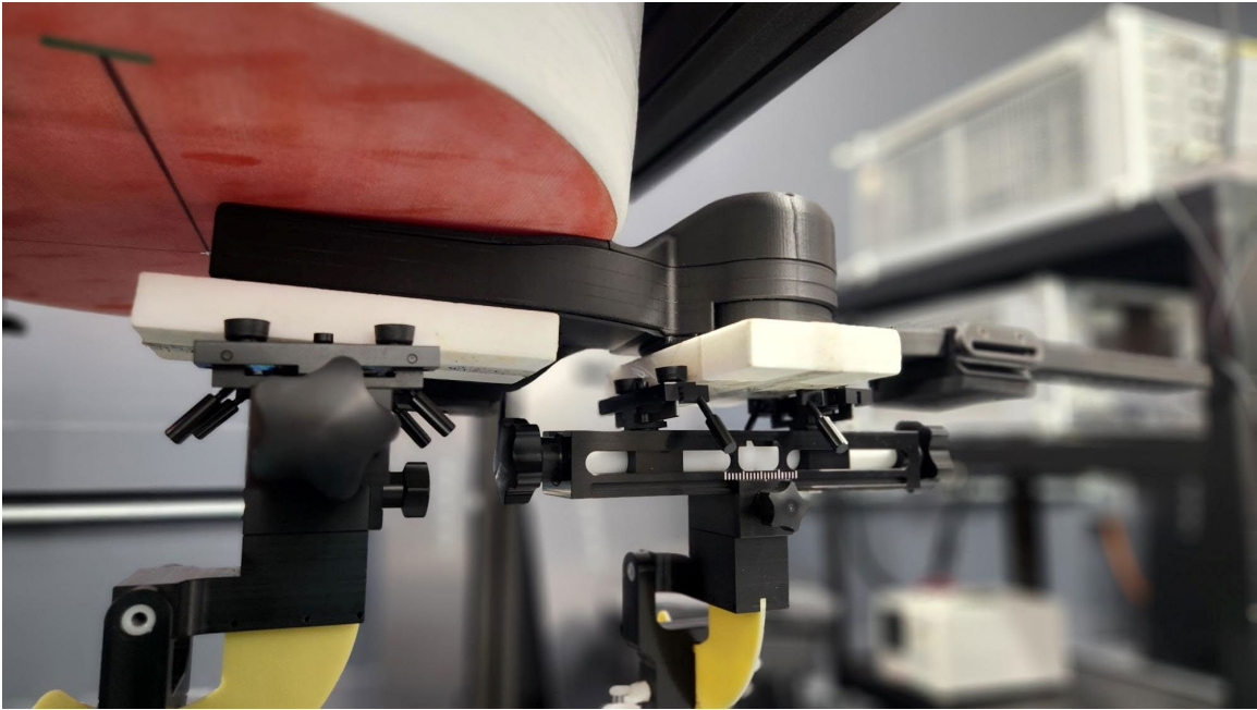
Figure C SAR Test Setup – Body – Front 0mm
