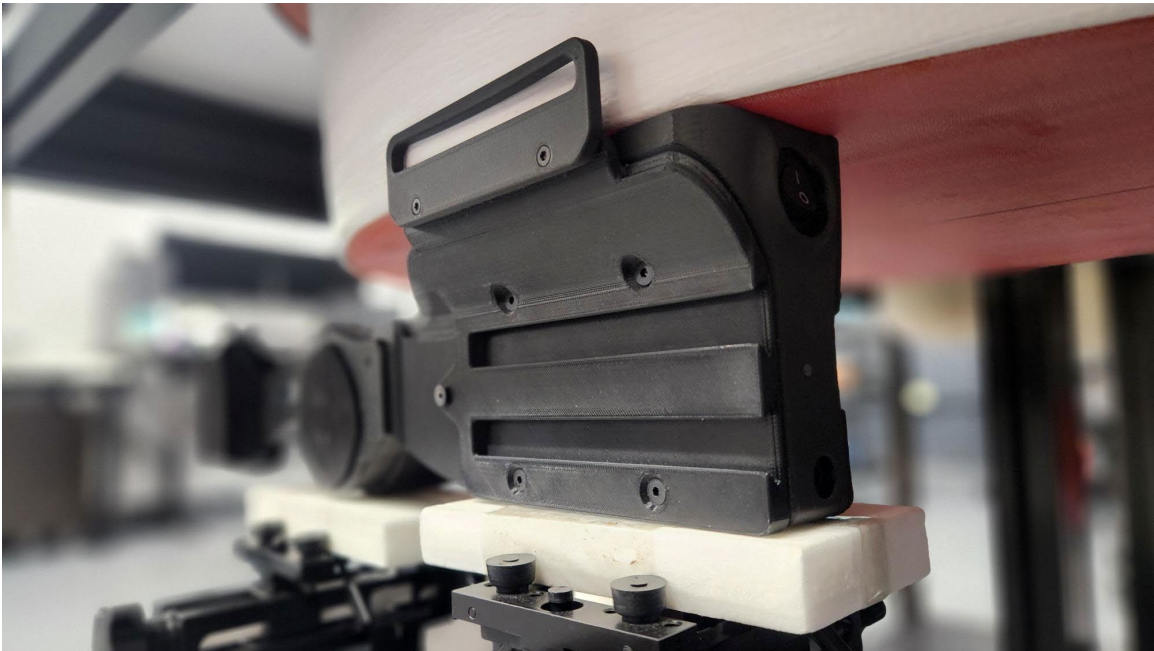
Figure D SAR Test Setup – Body – Top 0mm
