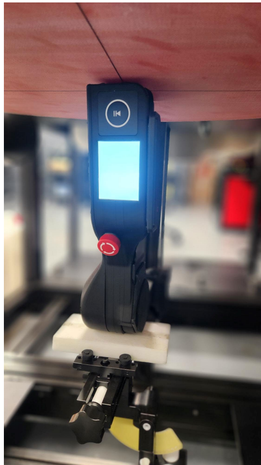
Figure F SAR Test Setup – Body – Left 0mm
