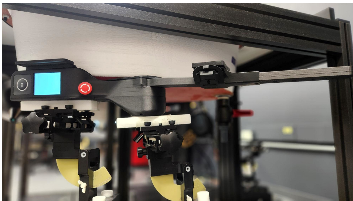
Figure B SAR Test Setup – Body – Back 0mm
