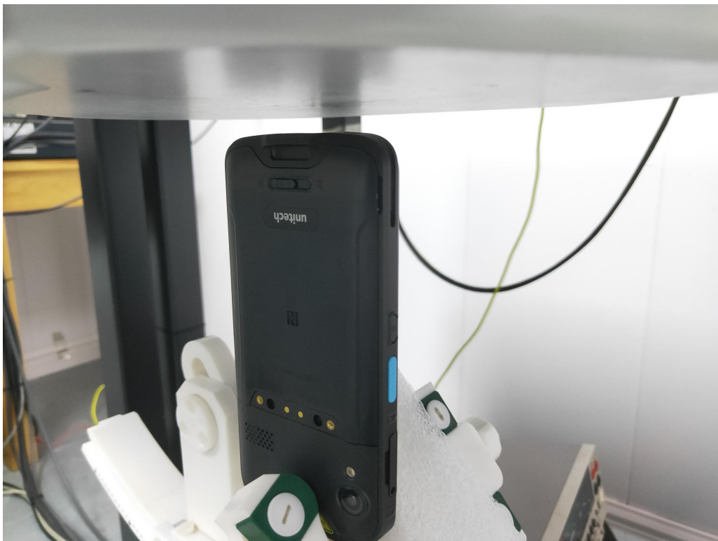
10mm body-worn Bottom Side Setup Photo (hotspot)
