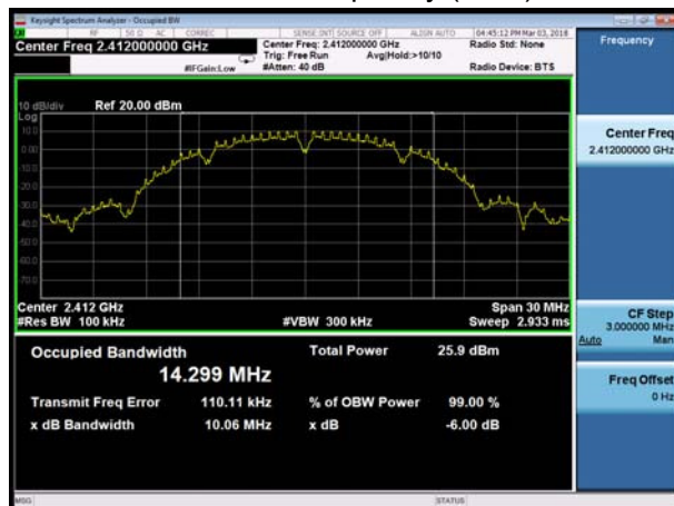
802.11b, Carrier frequency (MHz): 2437
