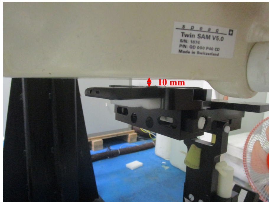
Body (Worn) Front Setup Photo (10mm)
