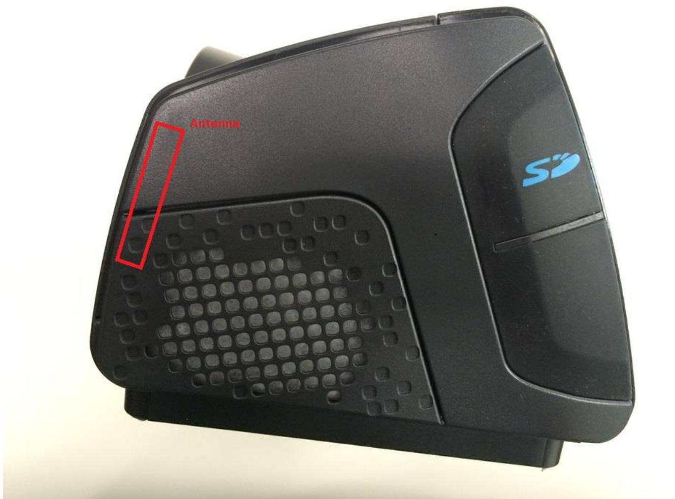
Cellular Antenna location
