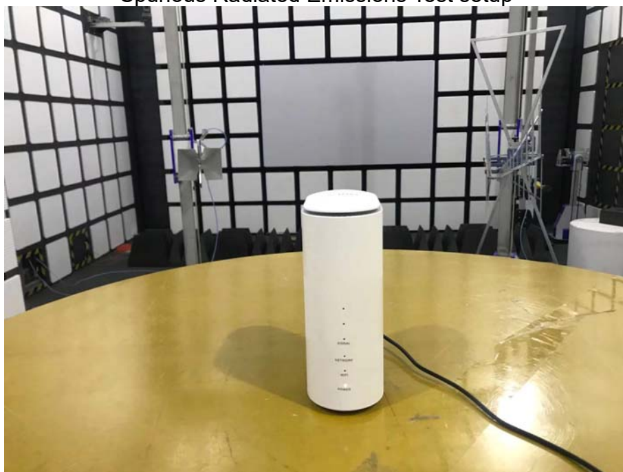
Spurious Radiated Emissions Test setup
