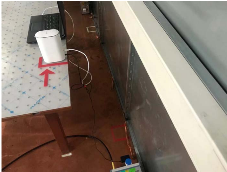
Conducted Emissions Test Setup (with charger)
