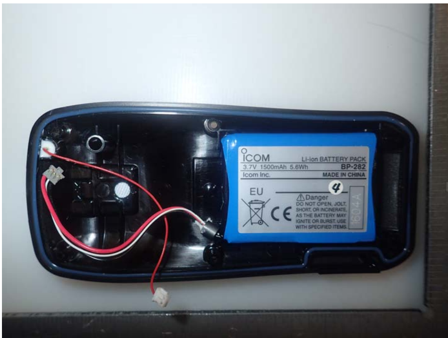
Li-ion Chargeable Battery (M/N: BP-282, 3.7V, 1500mAh)
