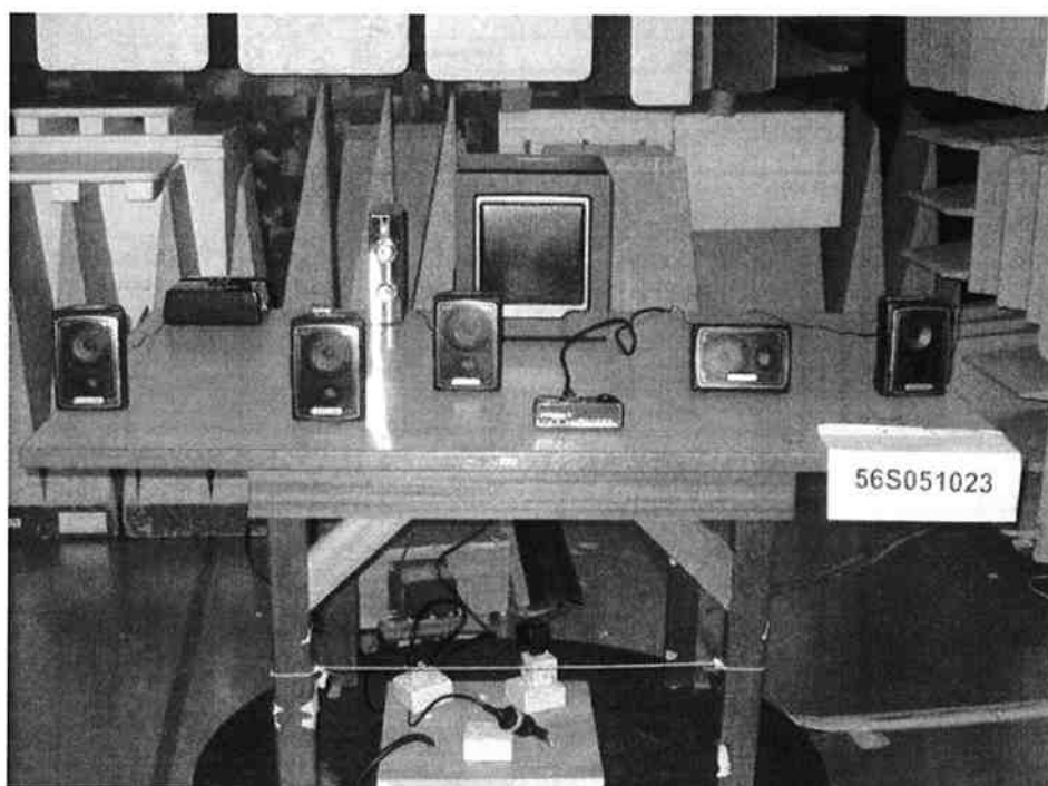
Radiated Emissions Test Setup (Front View)
