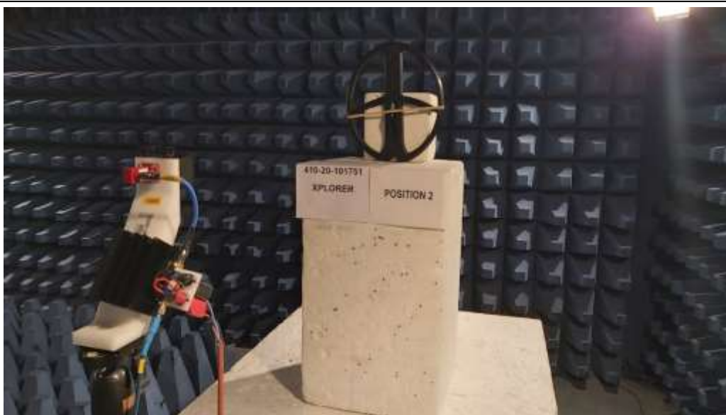
TEST SETUP PHOTO(S) - RX MODE / 18GHZ TO 26.5GHZ
