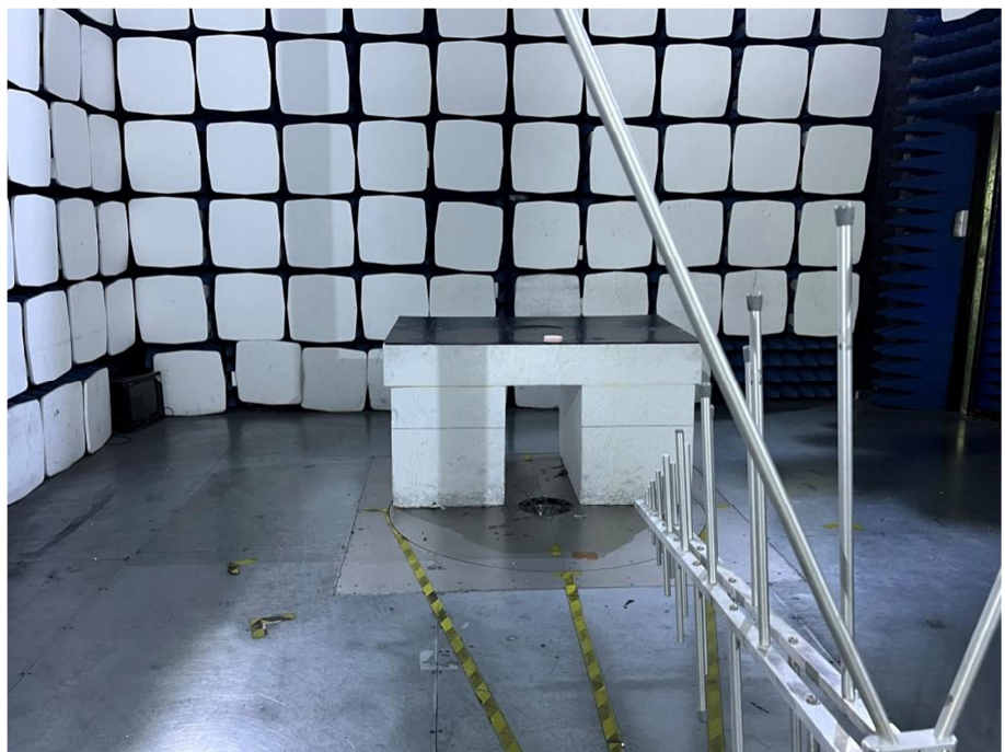
Radiation Emission Test Setup (30MHz to 1GHz)
