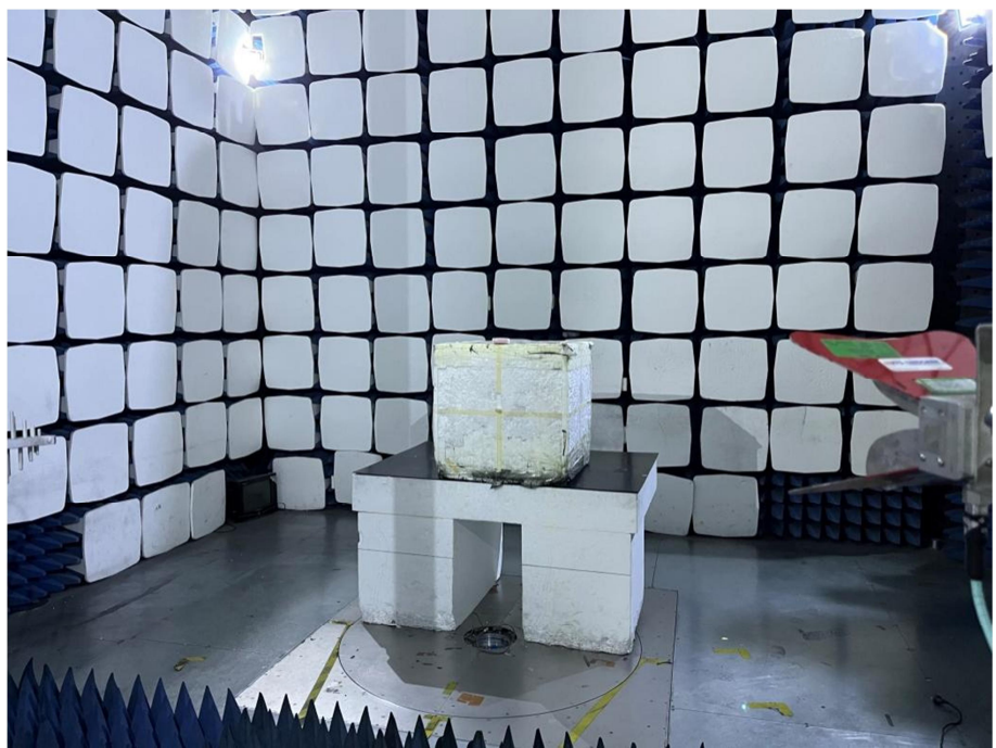
Radiation Emission Test Setup (1GHz to 18GHz)
