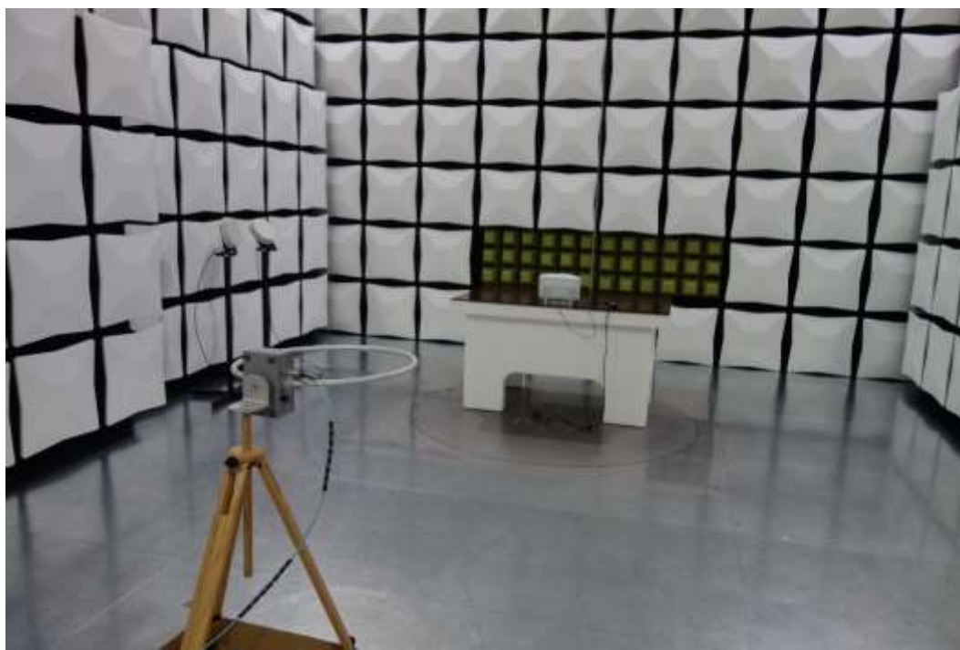
Antenna in parallel to floor position. Picture 1
