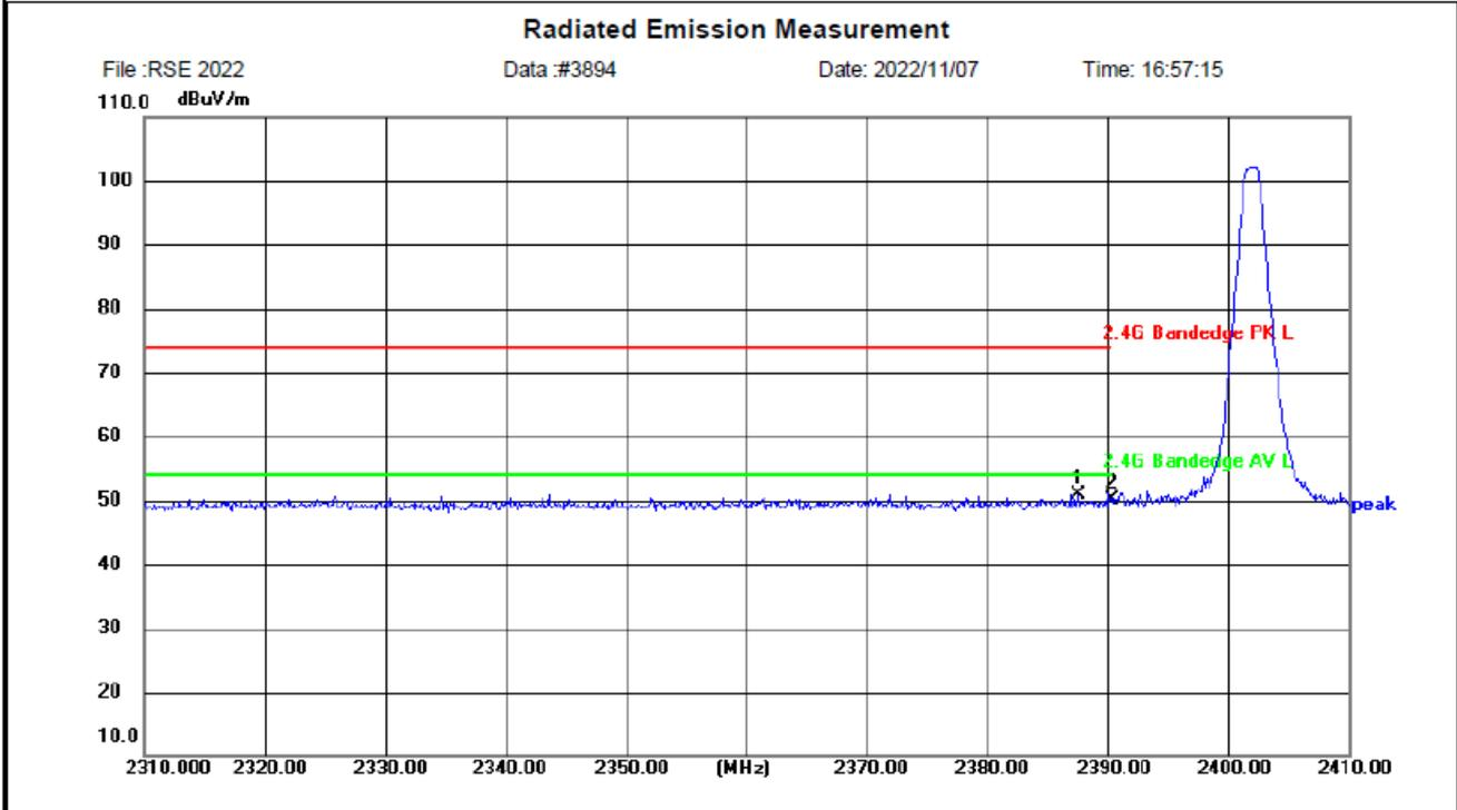
Site CTL 966 Chamber 1      Polarization: **Horizontal**      Temperature: 25(C)
