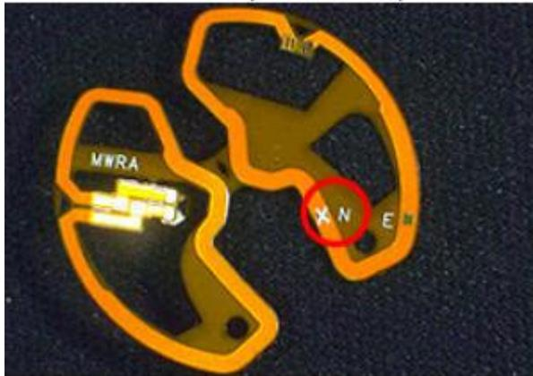
Fig.1 Picture of the antenna used in the Muse iQ R wireless hearing aid
