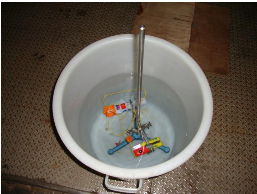
Test Set-up – Thermal Shock (submerged EUTs)
