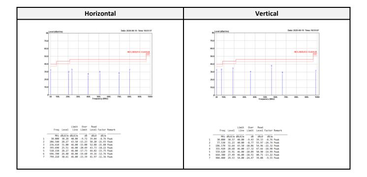
Level = Reading Level + Correct Factor
