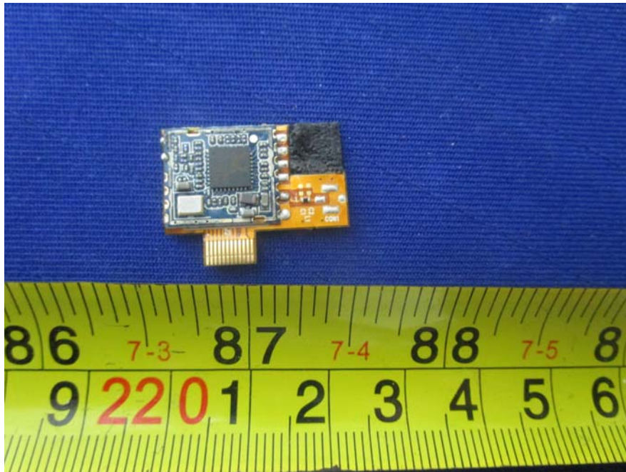
EUT – RF Board Top Unshielded View
