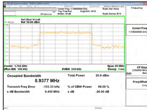
5G NR n66 10MHz BPSK Middle Channel RB50-0
