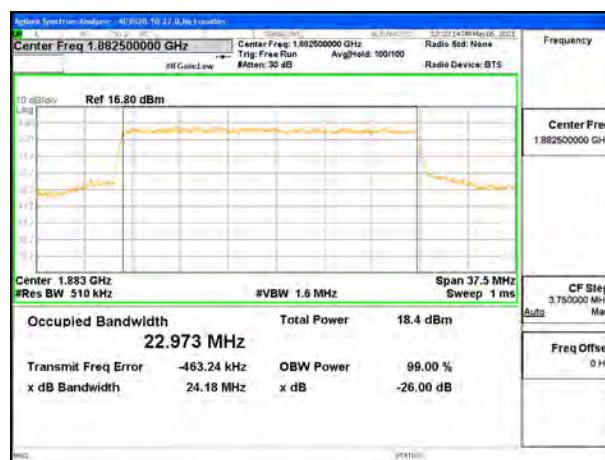
5G NR n25 25MHz BPSK Middle Channel RB128-0
