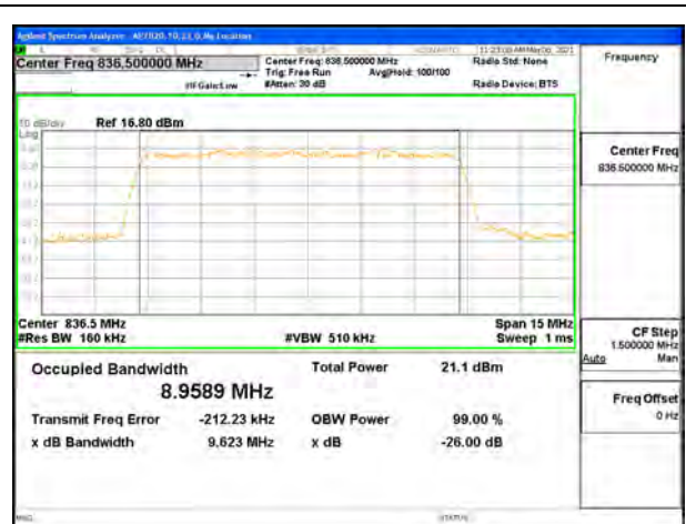
5G NR n5 10MHz BPSK Middle Channel RB50-0
