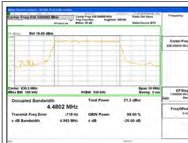
5G NR n5 5MHz BPSK Middle Channel RB25-0
