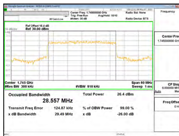
5G NR n66 30MHz BPSK Middle Channel RB160-0
