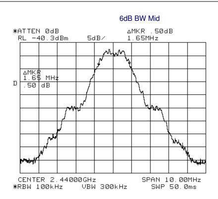
The 6 dB bandwidth for the mid frequency is 1.65 MHz.
