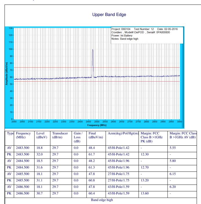
Band-edge should be -20 dBc (peak) and -30 dBc (average), or must comply with the limits of 15.209 if they fall in a restricted band.
