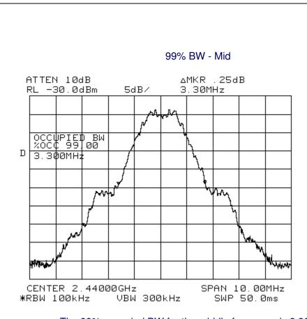
The 99% occupied BW for the middle frequency is 3.30 MHz.
