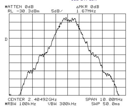
The 6 dB bandwidth for the low frequency is 1.67 MHz.
