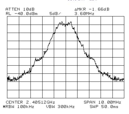
The 99% occupied BW for the lowest frequency is 3.60 MHz.
