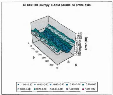
Probe isotropy for E<sub>tot</sub>: probe rotated  $\phi$  = 0° to 360°, tilted from field propagation direction  $\overline{k}$  Parallel to the field propagation ( $\psi$  =0° - 90°) at 30 GHz: deviation within ± 0.40 dB Parallel to the field propagation ( $\psi$  =0° - 90°) at 60 GHz: deviation within ± 0.40 dB
