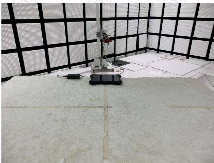
Radiated spurious emission Test Setup-2(Above 1GHz)
