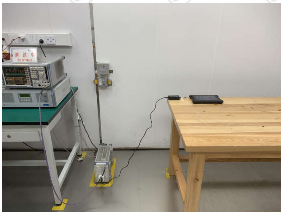
Conducted Emissions Test Setup
