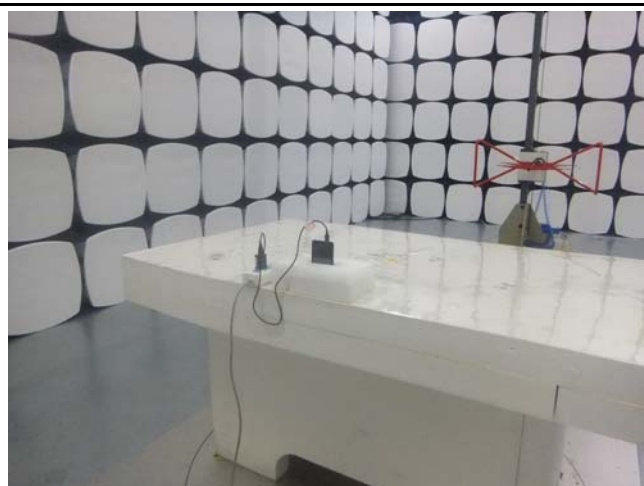
Conducted Emissions Test Setup Front View
