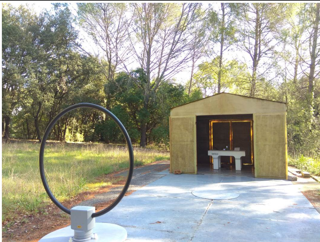
TEST SETUP PHOTO(S) RADIATED EMISSION( F < 30\text{MHz} , FINAL MEASUREMENT)
