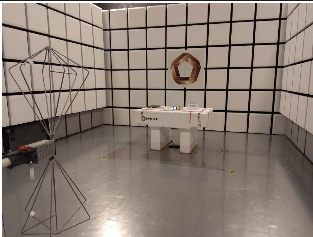
TEST SETUP PHOTO(S) RADIATED EMISSIONS (30MHz-200MHz)
