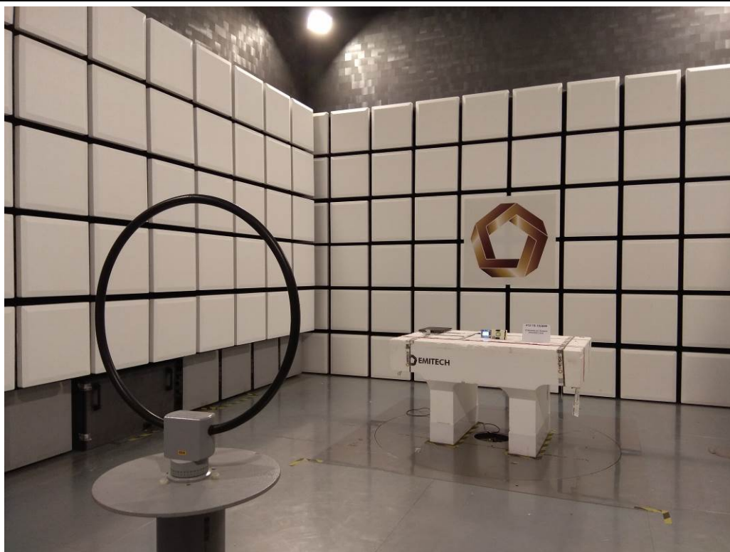
TEST SETUP PHOTO(S) RADIATED EMISSION( F < 30\text{MHz} , PRE MEASUREMENT)
