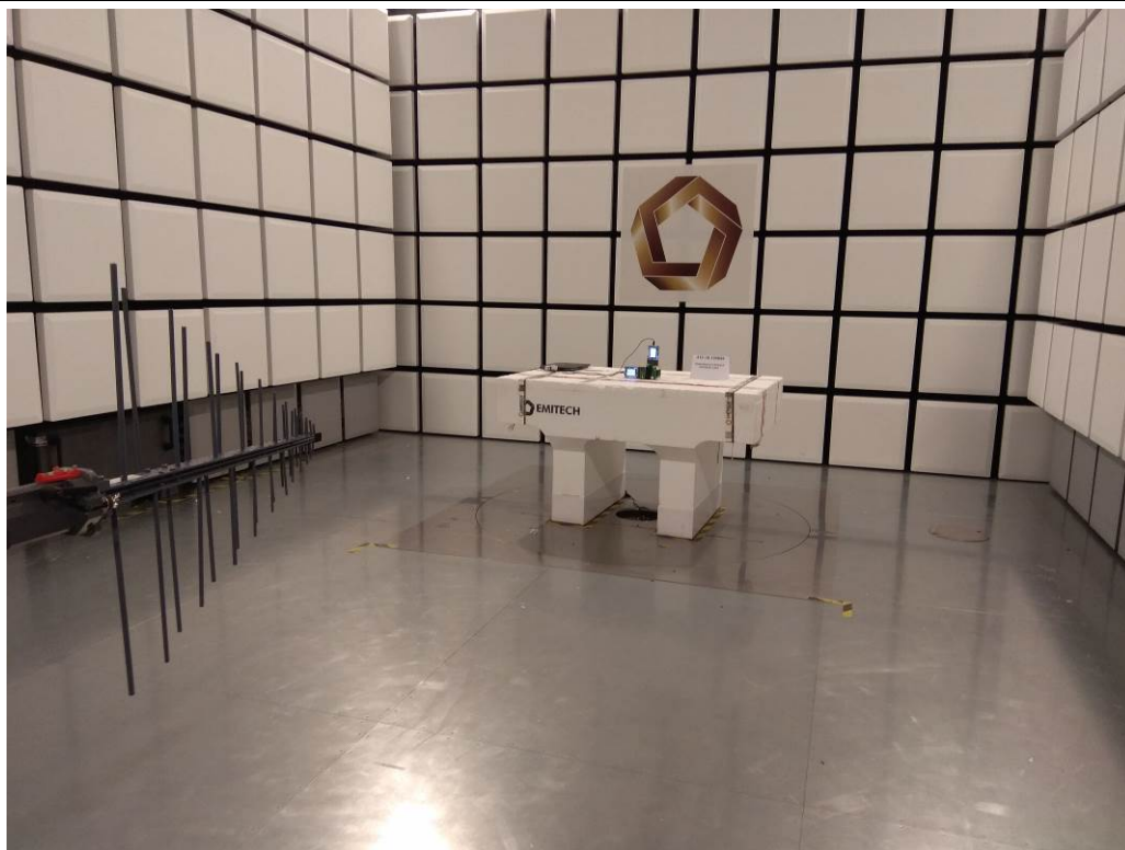
TEST SETUP PHOTO(S) RADIATED EMISSIONS (200MHz-1GHz)
