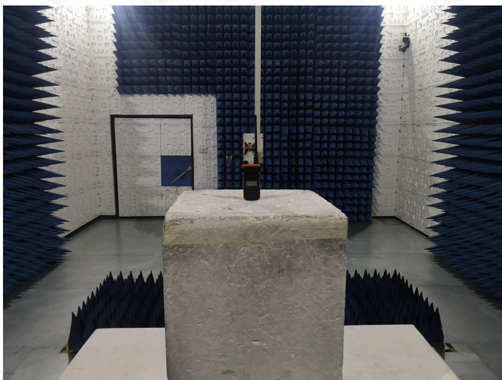
RADIATED EMISSION ABOVE 1G TEST SETUP
