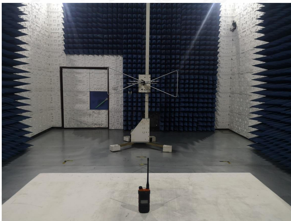
RADIATED EMISSION ABOVE 1G TEST SETUP
