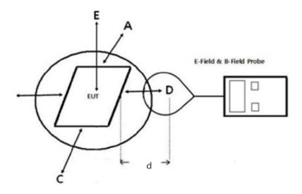
Note: Position A: Front of EUT; Position B: Left of EUT; Position C: back of EUT; Position D: Right of EUT; Position E: Top of EUT(20 cm measure distance);
