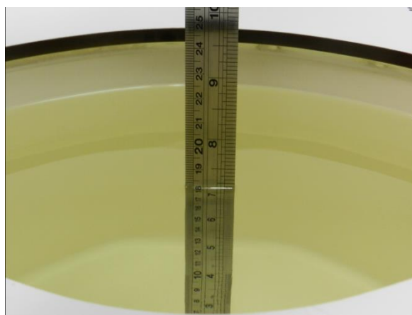
Fig 10.2 Photo of Liquid Height for Body SAR
