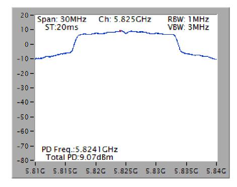
Power Density Plot on Configuration IEEE 802.11a / Ant. 1 + Ant. 2 / 5825 MHz
