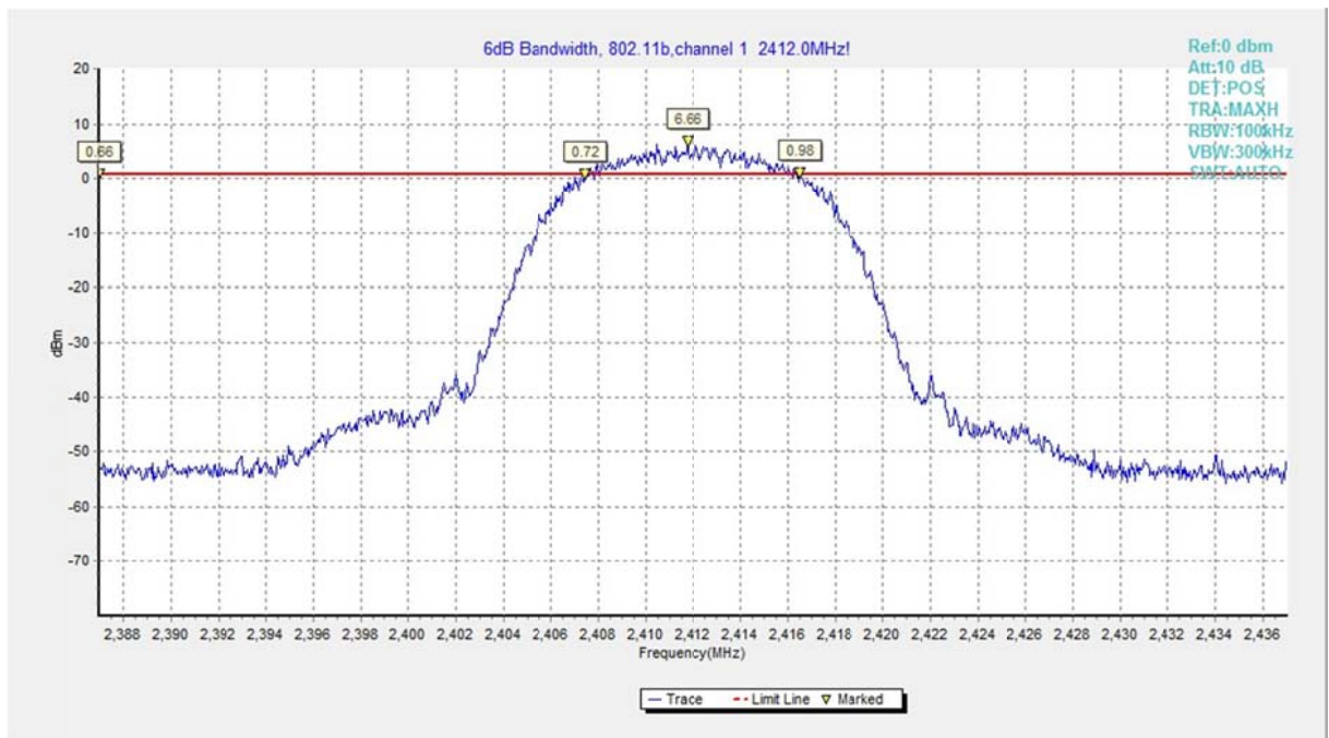
Fig.A.4.1 Occupied 6dB Bandwidth(802.11b,Ch 1)
