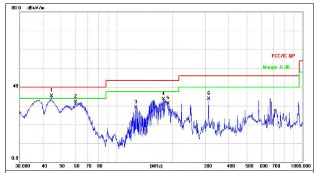
Remark: Factor = Antenna Factor + Cable Loss – Pre-amplifier.
