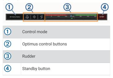
You must press a mode button on the overlay bar to engage or disengage the mode. When the mode is engaged, the button is illuminated.
