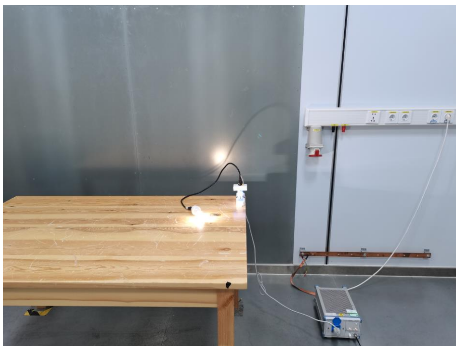
Fig. 4 Power line conducted emission setup photo
