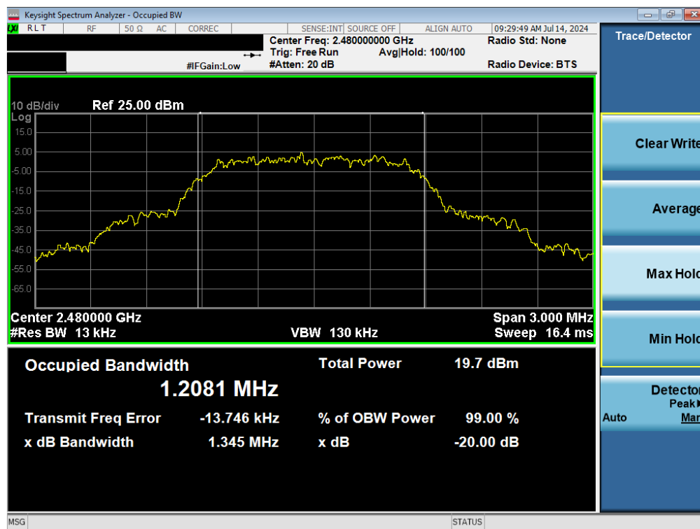
Plot 7-6. 20dB BW and 99% OBW Plot (Bluetooth, 8DPSK, ePA – Ch. 78)
