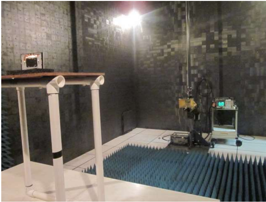
RADIATED EMISSIONS TEST SETUP 1 TO 18 GHZ
