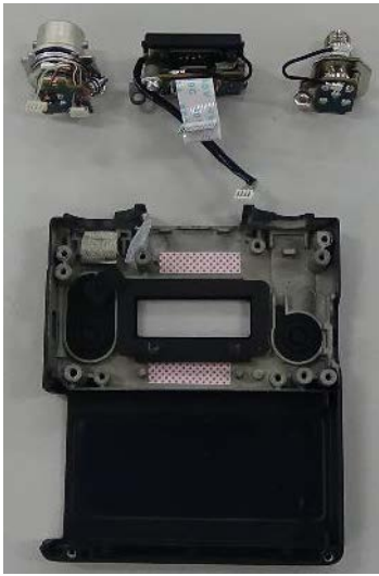
Fig.17:Remove the MIC/ANTENNA connector and RM assembly
