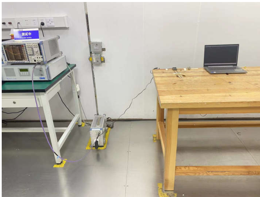
Conducted Emissions Test Setup-1
