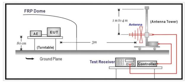
Above 1GHz Test Setup:
