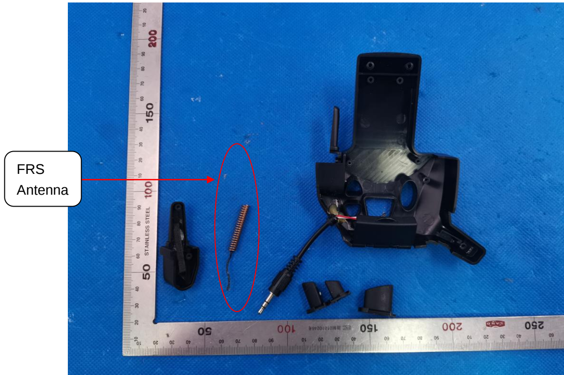
INTERNAL VIEW OF EUT (FIGURE 6)
