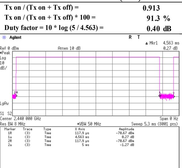
\* Since the burst rate is not different between the channels, the data has been obtained on the representative channel.
